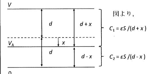
答  $C_1 = \frac{\epsilon S}{d+x}, \quad C_2 = \frac{\epsilon S}{d-x}$
